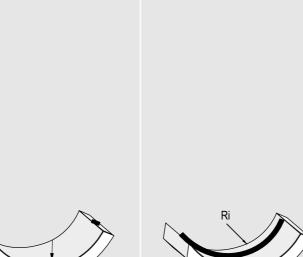
Brake lining inner radius (Ri) 40 mm ... 350 mm
